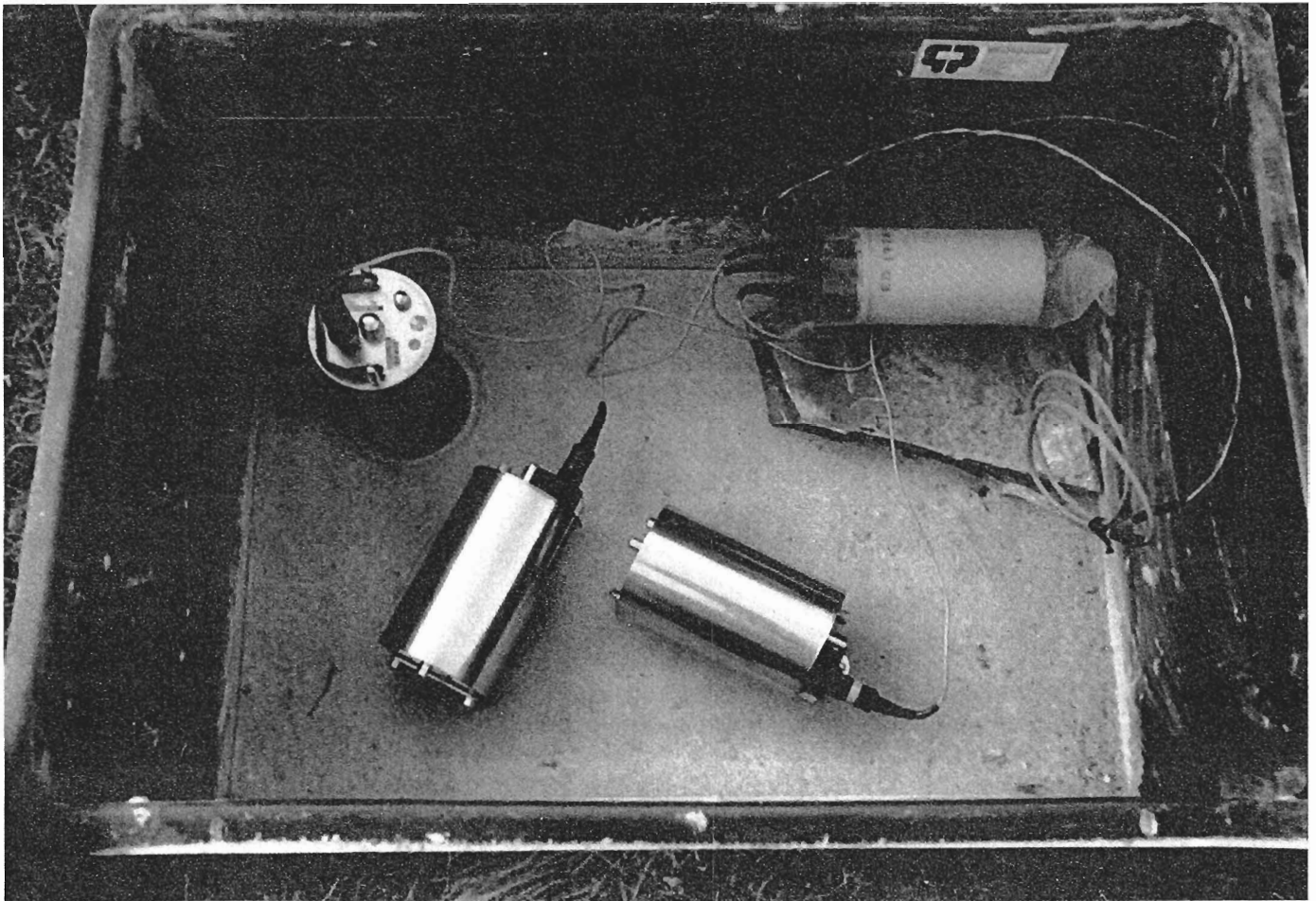
Above: A typical British Geological Survey three component seismometer pit
